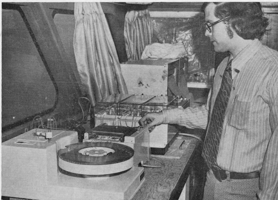
MICHAEL MCGUIRE studies a new auto-analyzer, which detects and measures chemical constituents of river water. The water is collected into tiny flasks of a sampler (left) and then is pumped to a module unit (middle). A colorimeter measures the constituents by intensity of color and the chart (photo at right) records the results.
