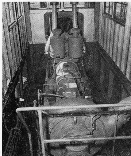
DREDGE OPERATOR manipulates long dredging "ladder" and revolving cutter from control booth. Pump at right can pump up to 4,000 gallons of sewage sludge per minute.
