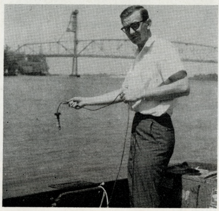
DISSOLVED OXYGEN IN THE DELAWARE RIVER is measured by Frederick L. Schaefer (left) and Thomas E. White, of the U. S. Geological Survey, with a new portable device. The sensitive cable and recorder, jointly tested by the Water Department and USGS, may reduce lab work and sampling personnel. For another development, see story at right.
