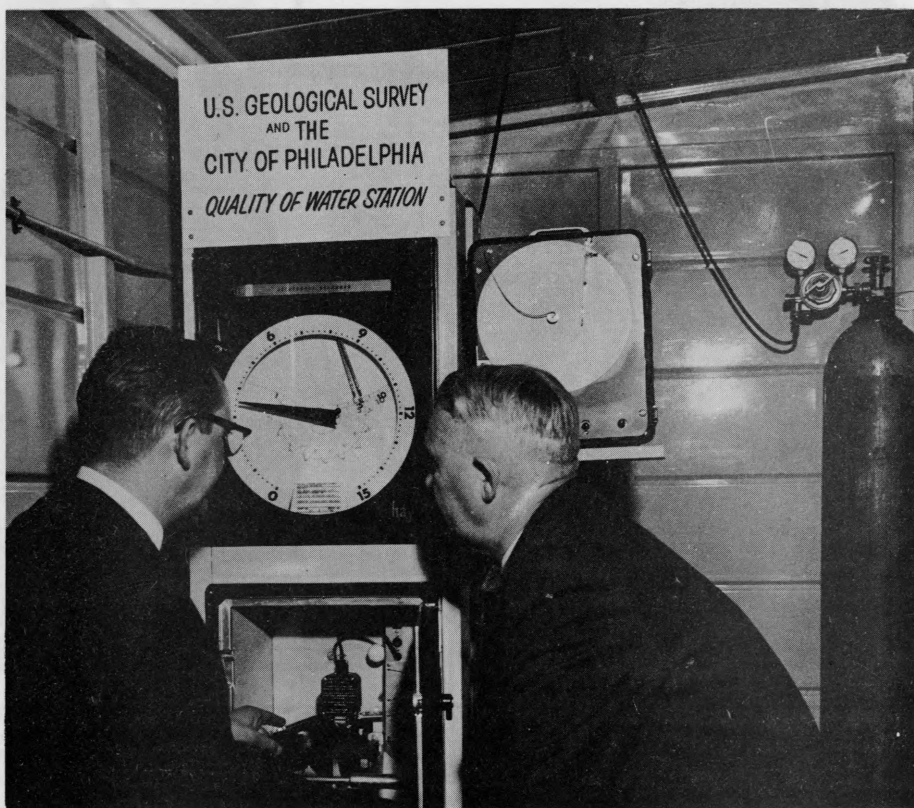
AN AUTOMATIC DETECTIVE now partially replaces Joseph Radziul, holding flask (above), as well as other humans, in monitoring the Delaware River for pollution. Joe, the department's research and development engineer, is making a "dissolved oxygen determination" on a water sample for the television camera man, but the electronic device (below), which Joe and Commissioner Samuel S. Baxter are eying, can do the same thing automatically 24 hours a day. SEE STORY AT RIGHT.
