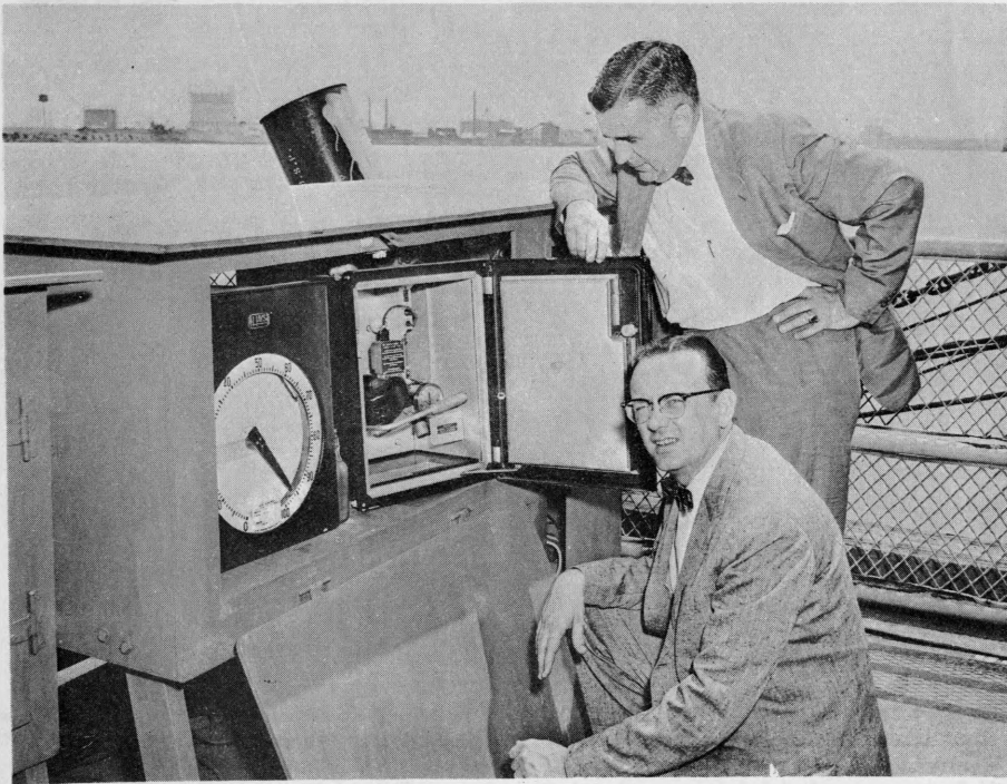
RIVER MONITORING EQUIPMENT is checked by Joseph V. Radziul (kneeling), who heads Water Department research and development, and Norman Beamer, chief chemist of U. S. Geological Survey. Equipment measures condition of Delaware River.
