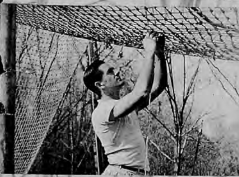
Constant repairs are needed on the safety net. It is inspected every time used, and here, Frank Longbottom, 1328 Howell st., makes a repair. Nets are handmade and may last for 20 years.
