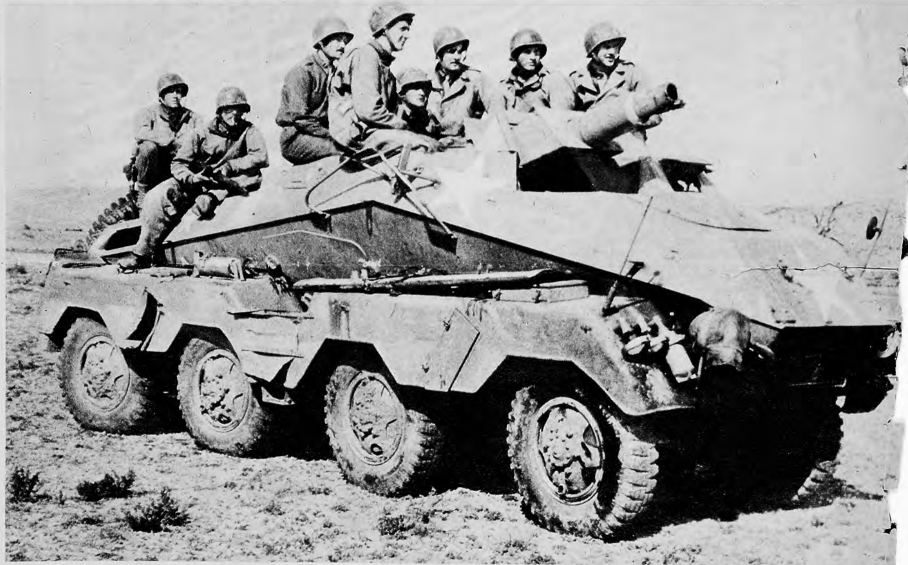
Prize piece of salvage is a German tank destroyer, now in use by the U. S. Army. It is armed with a howitzer, has dual controls for operation forward or backward.
