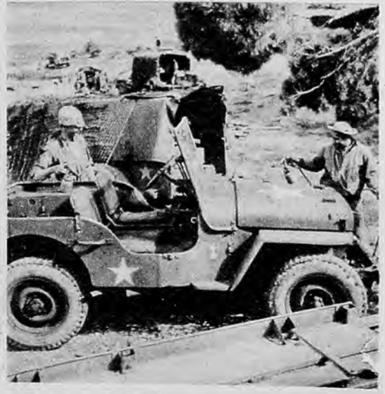
A jeep which had been put out of action by a mine receives a new coat of paint after undergoing repair by mechanics. Ordnance crews in salvage work are skilled in many trades.
