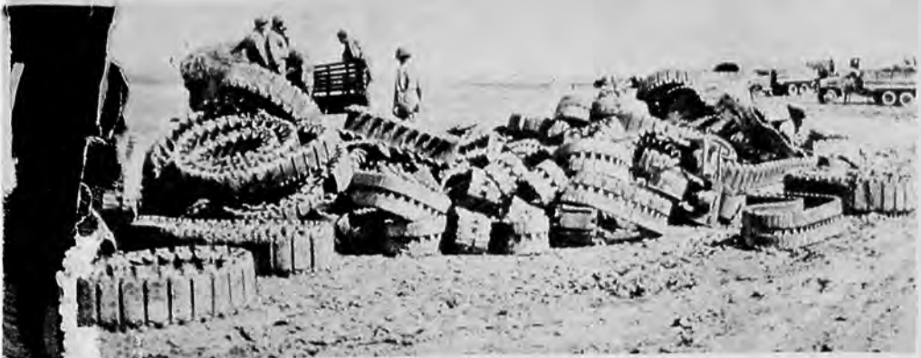
Treads from the battlefield are piled in huge heaps behind the lines to await repair. These serve as replacement parts, to be used on tanks or half-track vehicles whose treads have been battle-damaged beyond hope of recovery.
