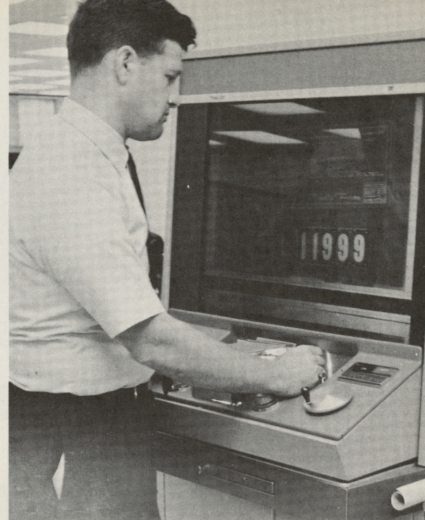
Management Aid: To its many items of modern business equipment, the Water Department added a machine for “reading” microfilmed records of engineering plans and reprinting copies of such plans from the microfilm. One result was the elimination of many filing cabinets for storage of cumbersome blueprints.
