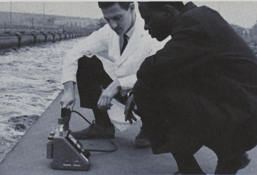
Water Pollution Control: The treatment of wastewater is constantly watched by laboratory personnel equipped with a variety of instruments. Portable recorder (photo) is used to check dissolved oxygen in plant aeration tanks.
