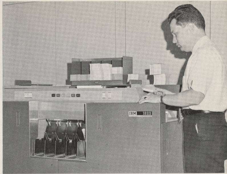
Engineering Computer Center: Ready to begin operation was a new office equipped with a computer capable of doing 100,000 calculations a minute. The computer, operated by the Water Department, will be used to solve quickly a variety of intricate engineering and planning problems that confront the department and other municipal agencies. Calculating unit at left; card read punch unit at right.
