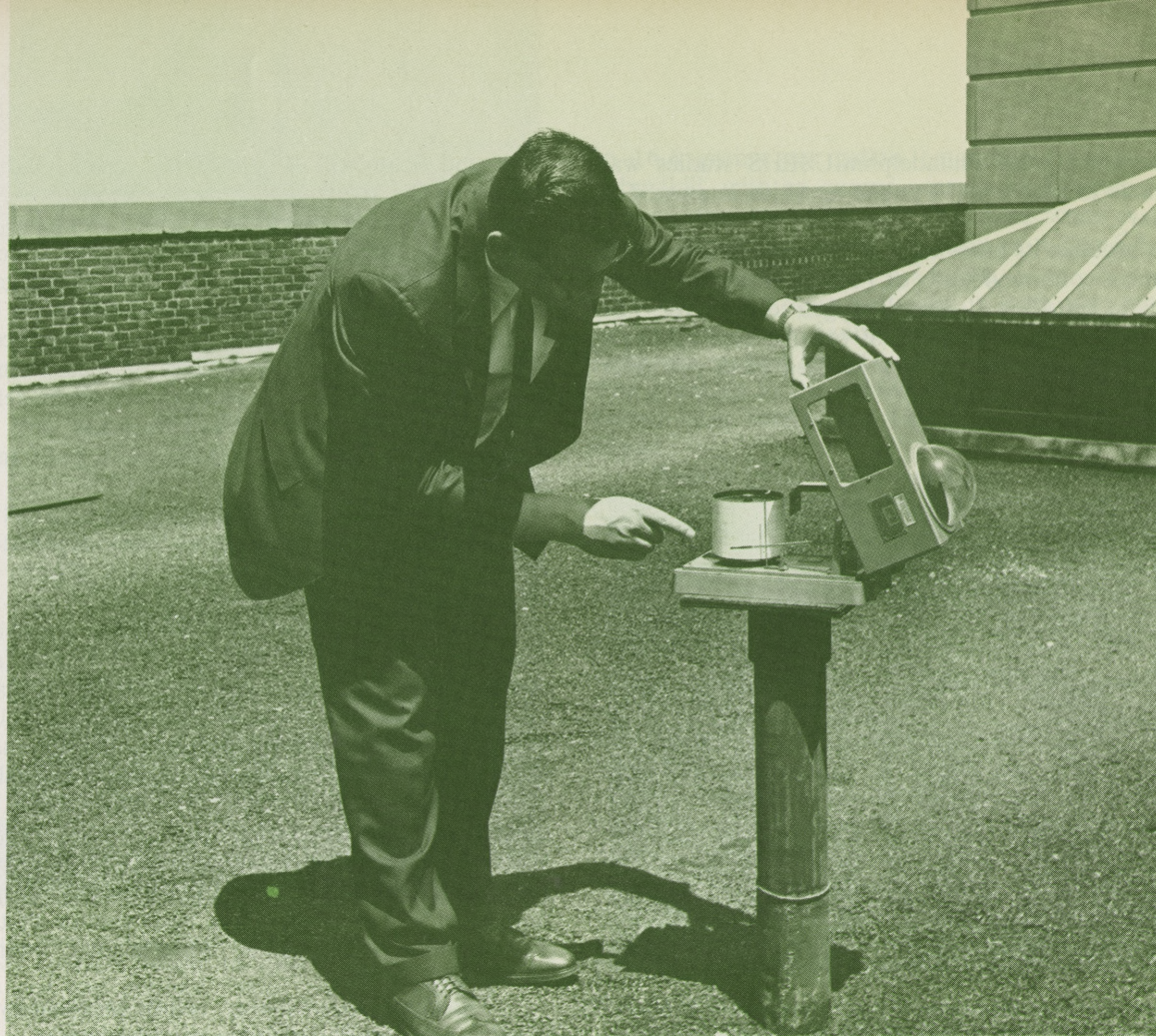
Photosynthesis Study: To learn more about the effect of sunlight on the growth of algae, which restore streams by releasing oxygen, the department acquired a portable pyroheliograph to measure sunlight intensity.
