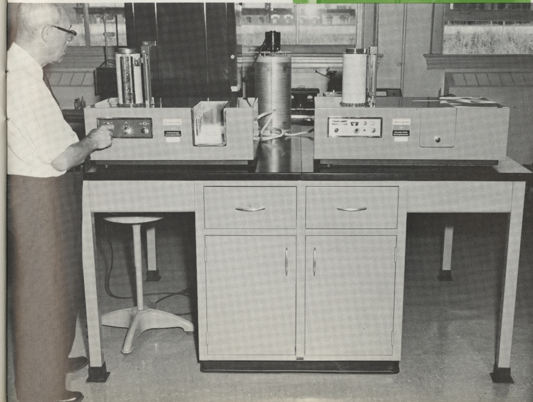
Electronic Detective: Infrared spectrophotometer is one of many sophisticated devices in the new quarters of the Materials Testing Laboratory. Spectrophotometer identifies new plastic materials.
