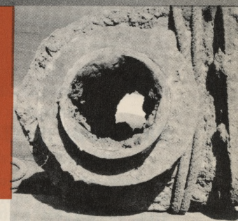
Pipe Cleaning: More than 13 miles of old water mains were cleaned and cement lined. Accumulation of sediment over years had cut down carrying capacity of some mains (see pipe sample at right).
