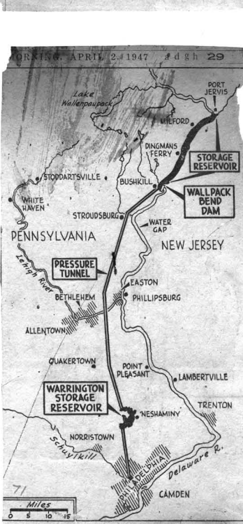
PROPOSED WATER SUPPLY FOR CITY The chart above shows in detail how the Wallpack Bend project would bring hundreds of millions of gallons of pure water daily to this city from the upper reaches of the Delaware River. Two huge reservoirs and an 81-mile-long pressure tunnel are features of the project.
