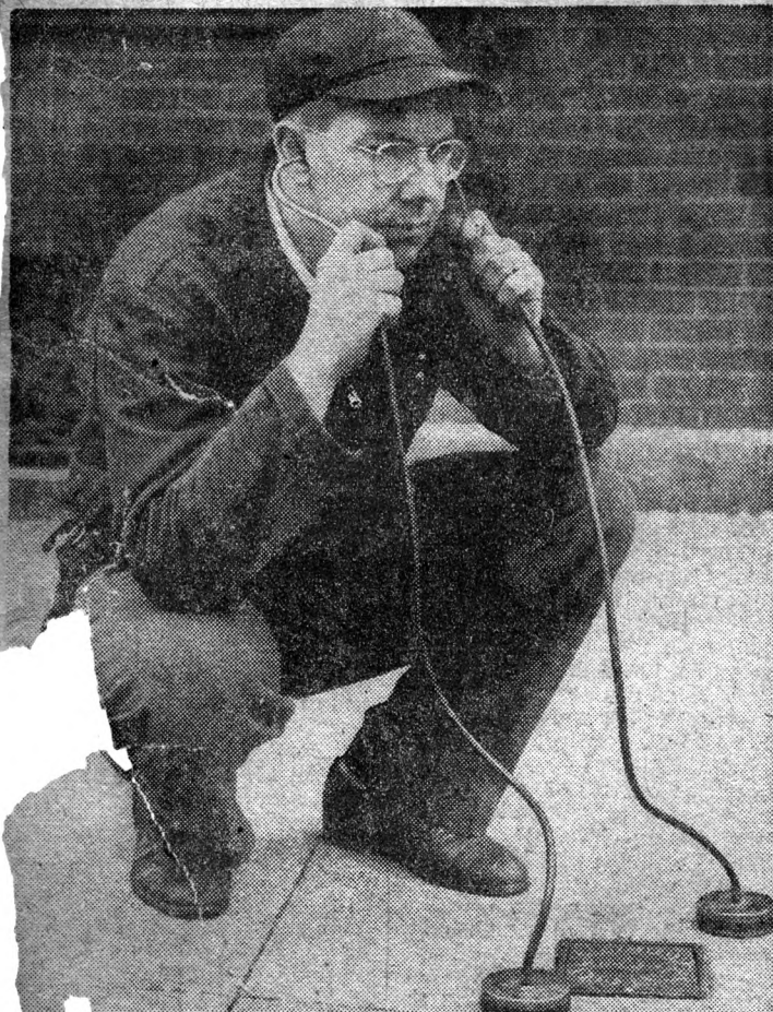
Kunder on the trail of a water main leak. He's in the Bureau of Water's leakage and waste survey. Instrument he's using is called a geophone.
