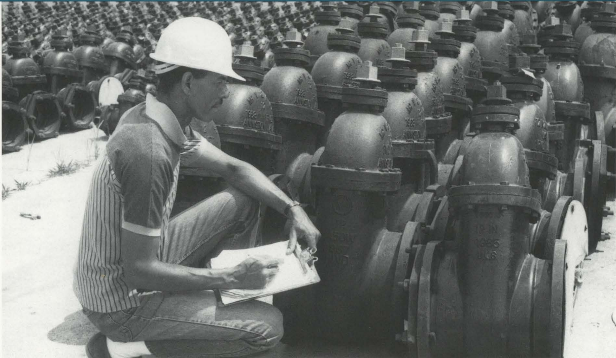
Foreman checks inventory of the 15,000 valves, ranging in size from three to forty-eight inches in diameter, ensuring that emergency repairs can be made to the water distribution system.
