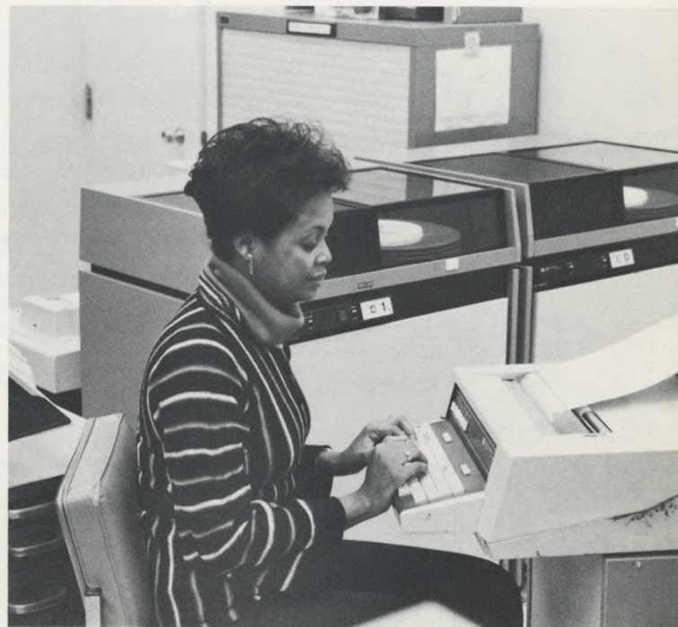
An employee at the Engineering Computer Center enters instructions on the HP 3000 acquired in 1975. Memory units in background each store up to 94 million characters. Secondary storage in the Center now totals 500 million characters.
