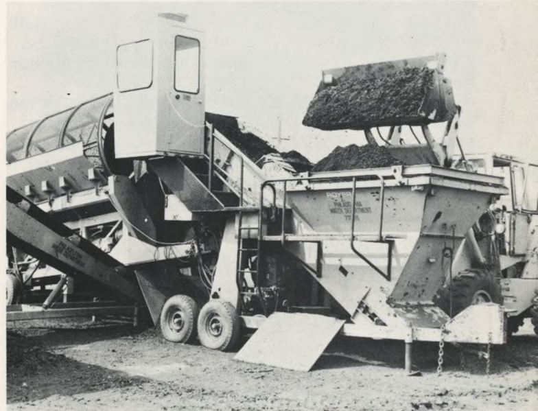
The composted sludge is screened to remove the bulking agent (wood chips) which is reused.
