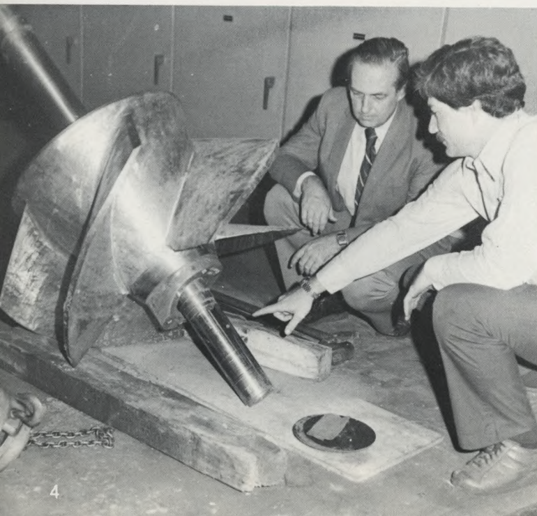
Stainless steel impeller for 60 MGD pump pulled for routine maintenance is inspected.
