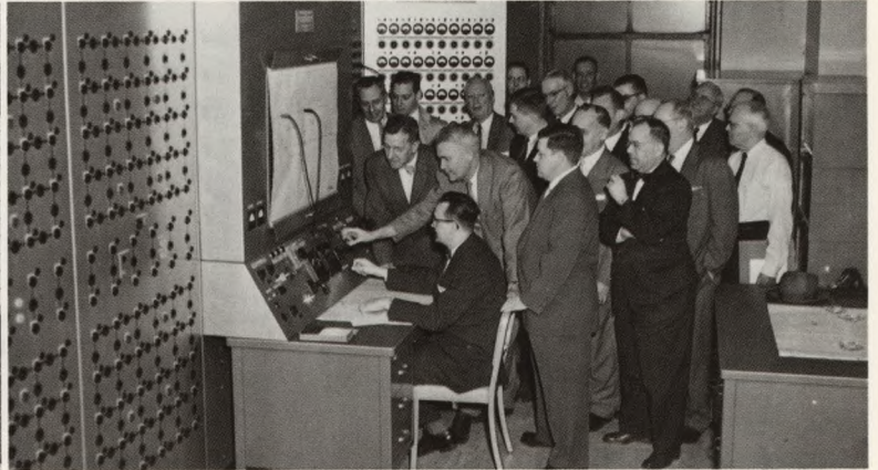
Back in the 1950's: The solution to many difficult problems in water flow was speeded up by the department's network fluid analyzer, sometimes called an analogue computer.
