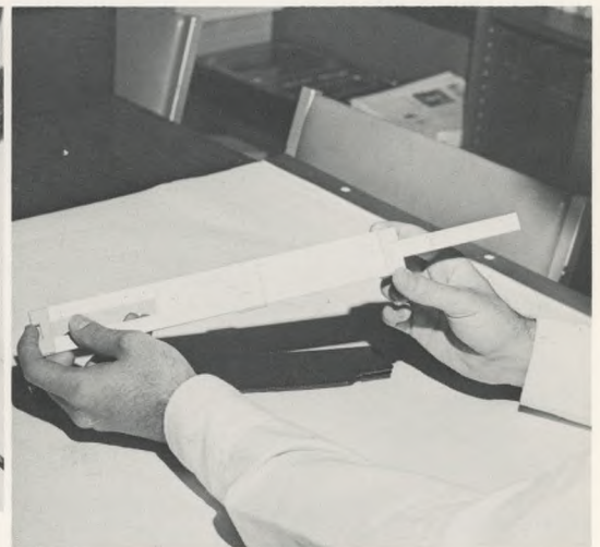
This Too Is History: At the turn of the century, city engineers used this complex revolving slide rule, which now reposes in the Water Department library. Today even a later simplified version has given way to small transistorized computers.
