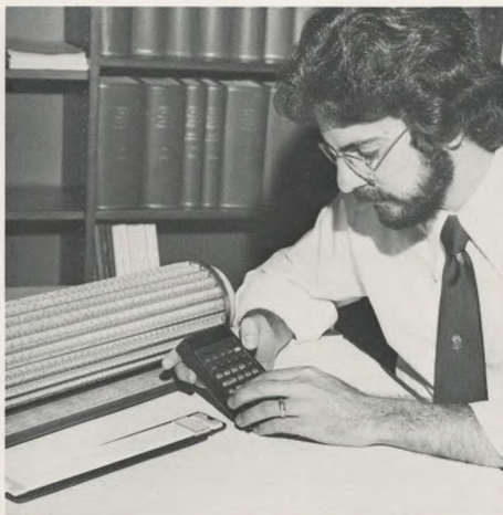
This Too Is History: At the turn of the century, city engineers used this complex revolving slide rule, which now reposes in the Water Department library. Today even a later simplified version has given way to small transistorized computers.
