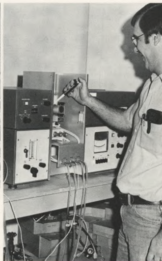
For Safe Ocean Disposal: Sludge barged to sea was carefully tested in Northeast laboratories. This chemist prepares a sludge sample and then screens it for heavy metals in an atomic absorption analyzer.
