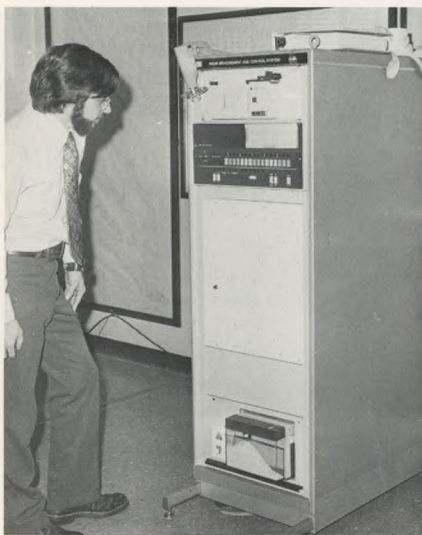
Computerizing Storm Overflow: To reduce future pollution of streams by storm sewers, the Water Department began to link 180 regulating chambers and 48 rain gauges to a new computer at the Northeast Plant.
