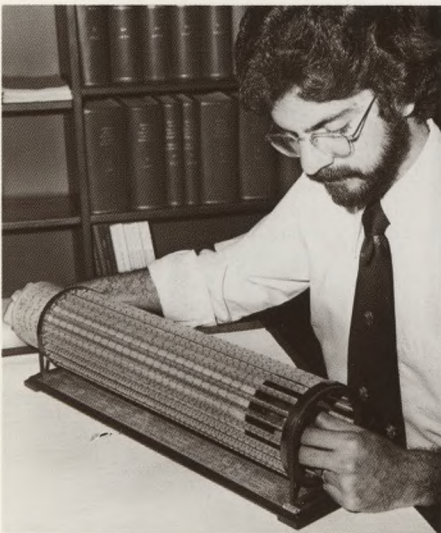
This Too Is History: At the turn of the century, city engineers used this complex revolving slide rule, which now reposes in the Water Department library. Today even a later simplified version has given way to small transistorized computers.
