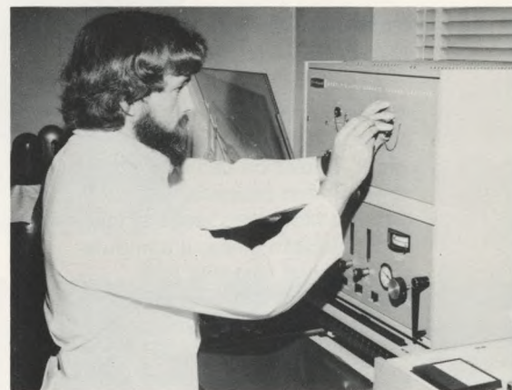
Automated Tests: Increasingly, plant laboratories were using automated equipment to speed up testing. At left, wastewater is deionized and filtered. Above, it is analyzed for total organic carbon.
