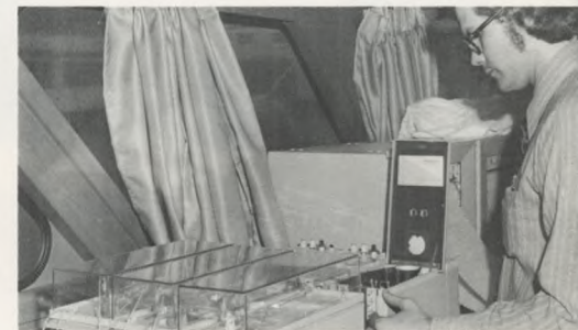
River Boat: In the onboard laboratory of the department's river boat, a new auto-analyzer sped up the analysis of river water. As the boat moved across the stream, water was collected into tiny flasks of a sampler (photos 1 and 2) and then was pumped to a module unit (photo 3). A colorimeter measured the constituents by intensity of color and the chart (photo 4) recorded the results.
