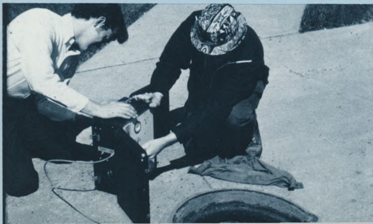
Waste Monitor: City engineers prepare to check an industry's wastes with an automatic sampler. An electric probe, inserted into a manhole sampling chamber, will trigger readings on the device.
