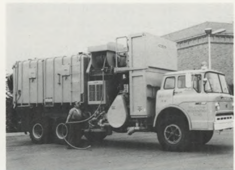
Vector Jets: Several “vector jets” were acquired for the first time to improve the cleaning of sewer inlets. Each vehicle combines a vacuum cleaning tube (left) with a high-pressure water jet hose (right) and related equipment.
