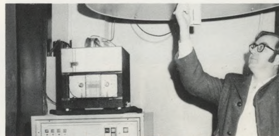
Link to Space: An engineer checks a disk antenna which relays data on the quality of river water to a space satellite. Stream monitoring unit at left.
