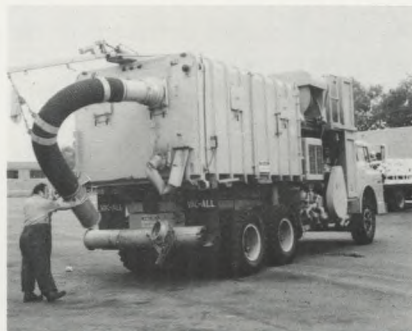
Vector Jets: Several “vector jets” were acquired for the first time to improve the cleaning of sewer inlets. Each vehicle combines a vacuum cleaning tube (left) with a high-pressure water jet hose (right) and related equipment.
