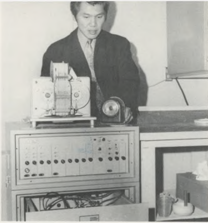
Stream Monitoring: Electronic equipment at eight stations keeps 24-hour vigilance over the Delaware and Schuylkill Rivers for the Water Department. This equipment analyzes and records dissolved oxygen, "pH", temperature, and other conditions of the river water.
