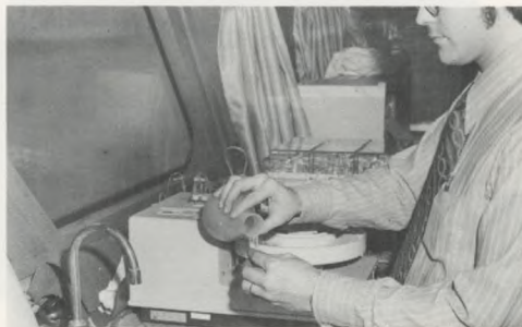
River Boat: In the onboard laboratory of the department's river boat, a new auto-analyzer sped up the analysis of river water. As the boat moved across the stream, water was collected into tiny flasks of a sampler (photos 1 and 2) and then was pumped to a module unit (photo 3). A colorimeter measured the constituents by intensity of color and the chart (photo 4) recorded the results.
