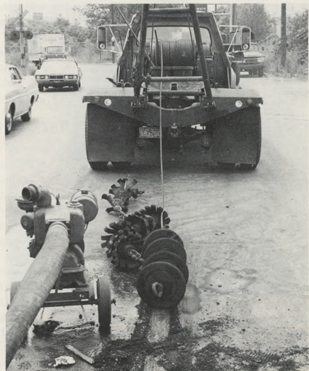
Cleaning Equipment: The city cleaned and cement lined 34 miles of old water mains during the biennium. Cleaning scrapers, which are pulled through mains by cable, together with flushing line and cable truck are shown above.
