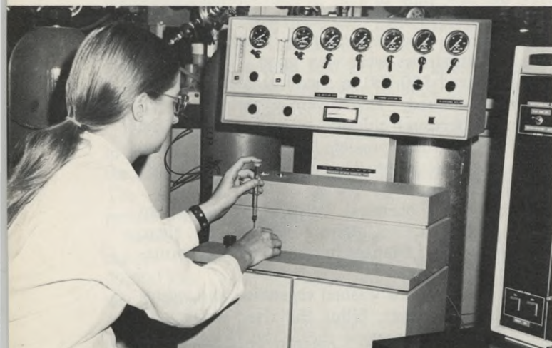
Automatic Testing Equipment: Acquired in 1970-71, this gas chromatograph is among many new automatic instruments introduced into Water Department laboratories. Such instruments eliminate many tedious wet chemical tests, while assuring faster and more continuous testing of the city's water.
