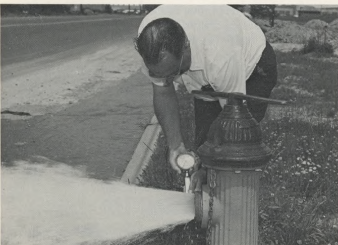
Checking Water Pressure: To make sure of adequate flow in event of fire, a supervisor checks the outpour of a hydrant. The blade of the delicate measuring instrument is placed against the flow, and the dial shows the pressure in pounds per square inch.
