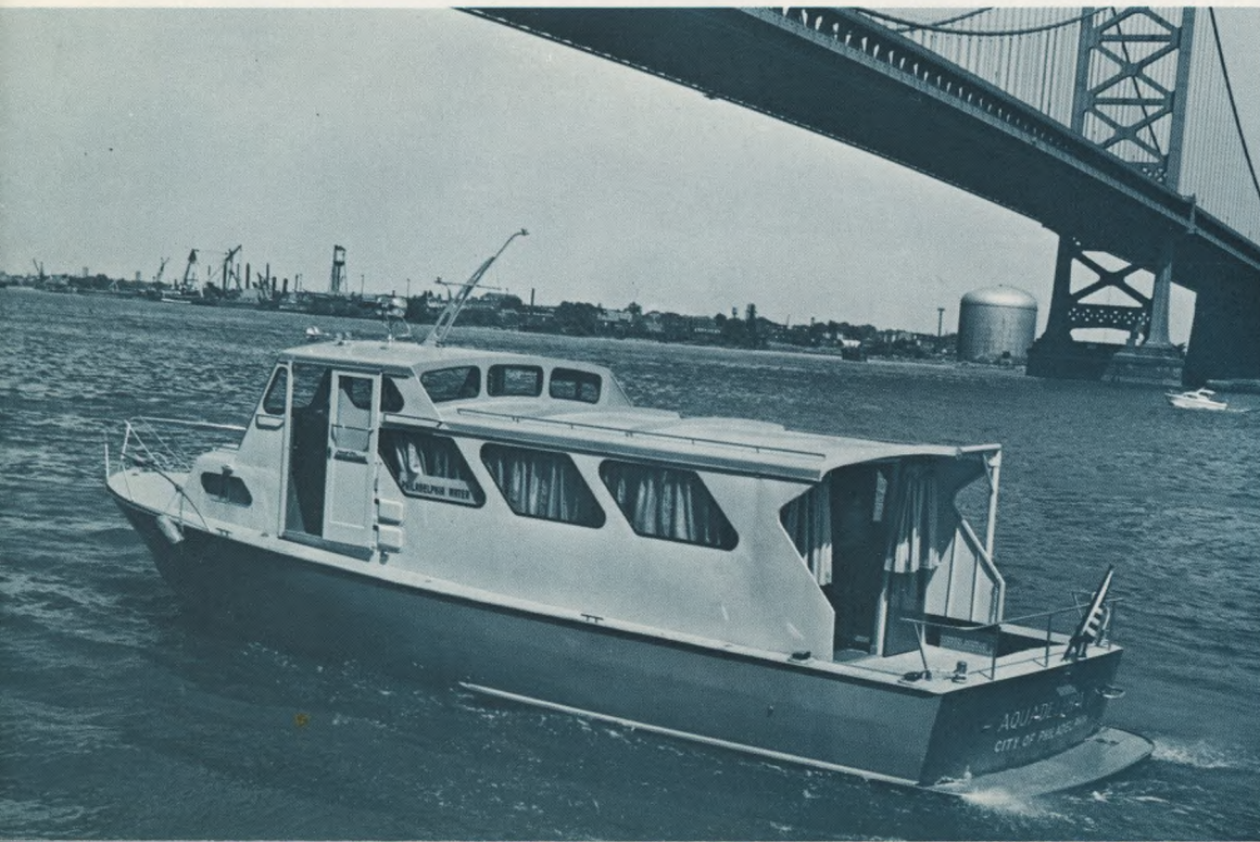
For River Study: Capable of 19 knots, this speedy cabin cruiser will improve the Water Department's study of the Delaware River estuary. The cruiser, delivered in 1969, makes possible the collection of water samples from all parts of the river.
