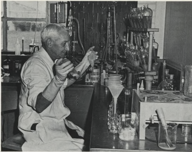
Unending Research: Plant chemists and sanitary engineers made 2.5 million tests on water samples, collected from rivers and from every point in the distribution system. At the Water Quality Research Laboratory, much attention was given to water odors, in the hope of finding new methods of control.
