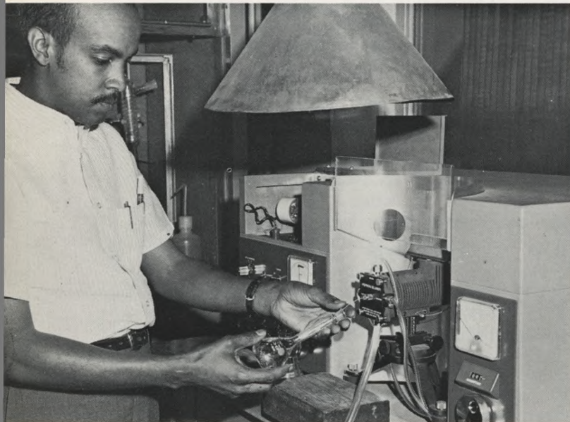
Laboratory Tests: To assure sound treatment, wastewater is sampled and tested at every stage as it flows through the water pollution control plants. In the two-year period, 1968-69, the plant laboratories made 400,000 tests on 100,000 wastewater samples.
