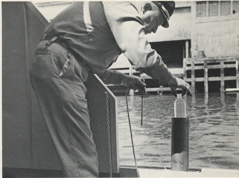
On-board Analyses: Equipped with an on-board laboratory (photo below), the department's new cabin cruiser allows sanitary engineers to study river water samples while afloat. Samples are drawn through the bottom of the boat, flowing out through laboratory faucets, or they are collected by brass container and bottle dropped overboard, as shown above.
