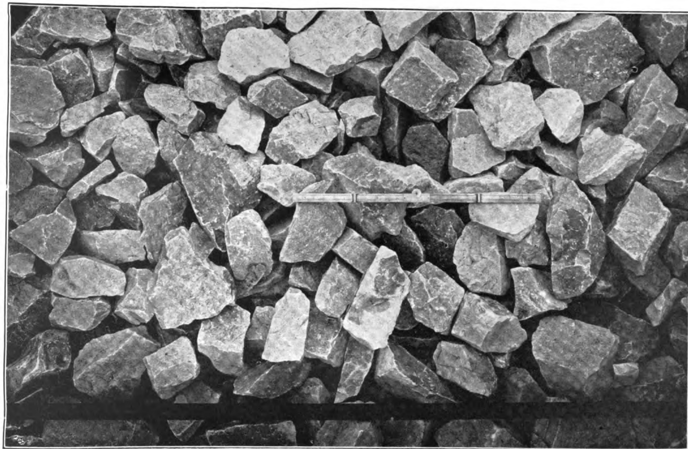
OUTSIDE SPRINKLING FILTER.—Station No. 20-2. 2½-inch to 4-inch limestone media.
